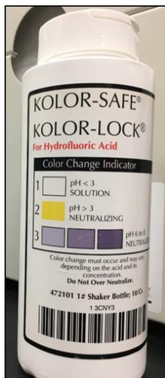
**Figure 8.4 Kolor-Safe® / Kolor-Lock® Solidifier** for hydrofluoric acid neutralization
